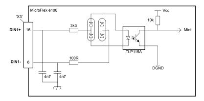
Figure 28 - General purpose fast digital input circuit
